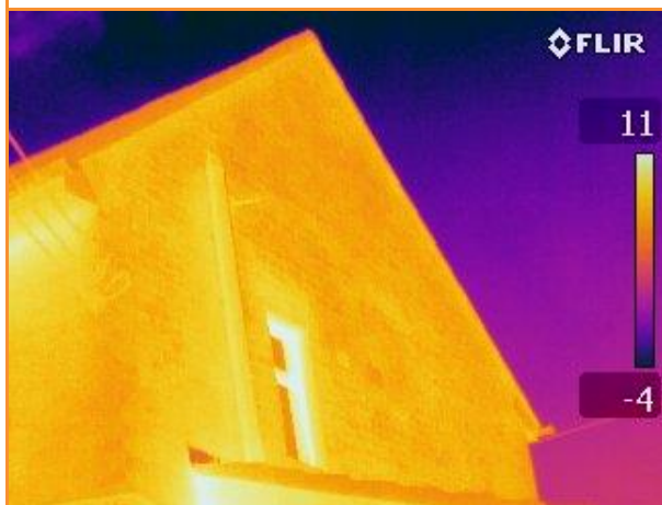
9.15: Thermographic image showing some leakage along the edge of the gable end
