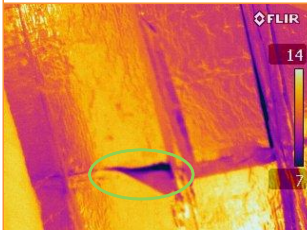
9.38: Thermographic image showing leakage past section of foil tape that has peeled off, building depressurised
