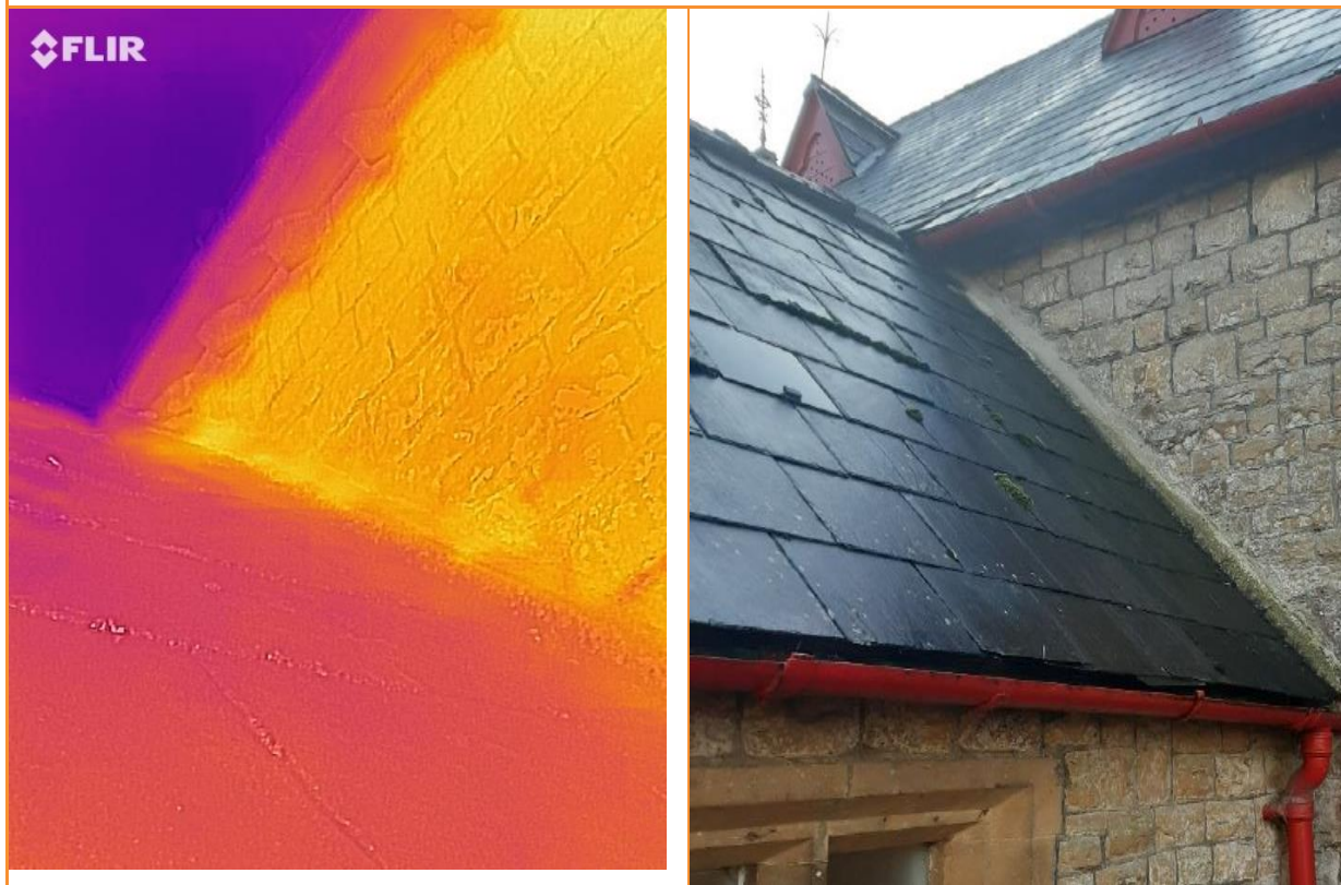
9.09: External thermographic image whilst building pressurised, showing warm air (white/yellow) escaping along (1) the sloping verge at the end of the entrance section and (2) the bottom edge of the main hall eaves
