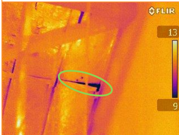
9.32: Thermographic image showing substantial leakage along eaves, whilst building pressurised
