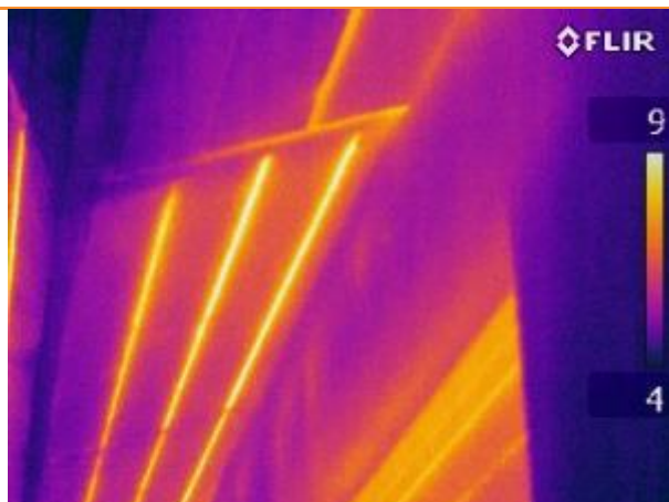
9.01: External thermographic image whilst house is pressurised showing leakage along section of eaves junction to top of wall above garage doorway.
